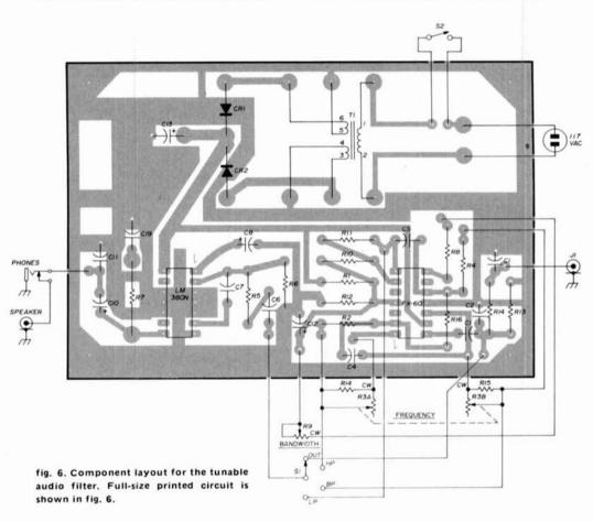
cations receiver. The output is then connected to the speaker or headphones and the filter can be switched into the circuit as required. The LM38ON provides two watts of audio output, more than enough for most applications.
